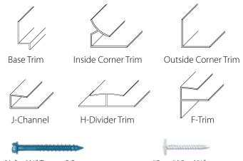
3/16" x 11/4" Tapcon® Screw with a stainless steel washer (1/4" ID. x 1/2" OD. x 1/32" thick) (supplied by others) #8 or #10 x 1¼" Stainless Steel Screw with ½" dia. low profile screw head (supplied by others)
