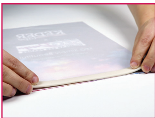
Apply KederTape to edges of fabric
